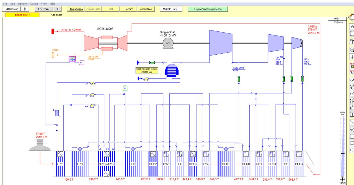
**THERMOFLEX** provides the **GT PRO®** gas turbine library and a reciprocating gas and diesel engine library which in the latest Version includes more than **700 gas turbine and 380 gas/diesel engine specifications**. The **Steam Turbine Assembly** feature provides automatic estimation of efficiencies, leakage flows and information about the entire steam turbine such as dimensions, weight and costs.
